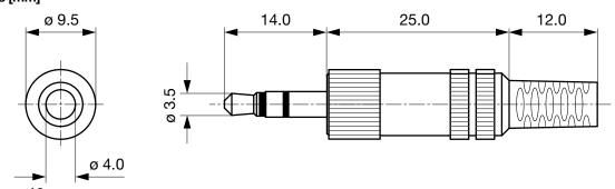
Cable diameter max. 4.0 mm
