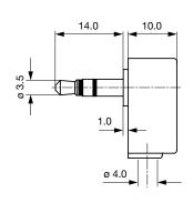
Cable diameter max. 4.0 mm
